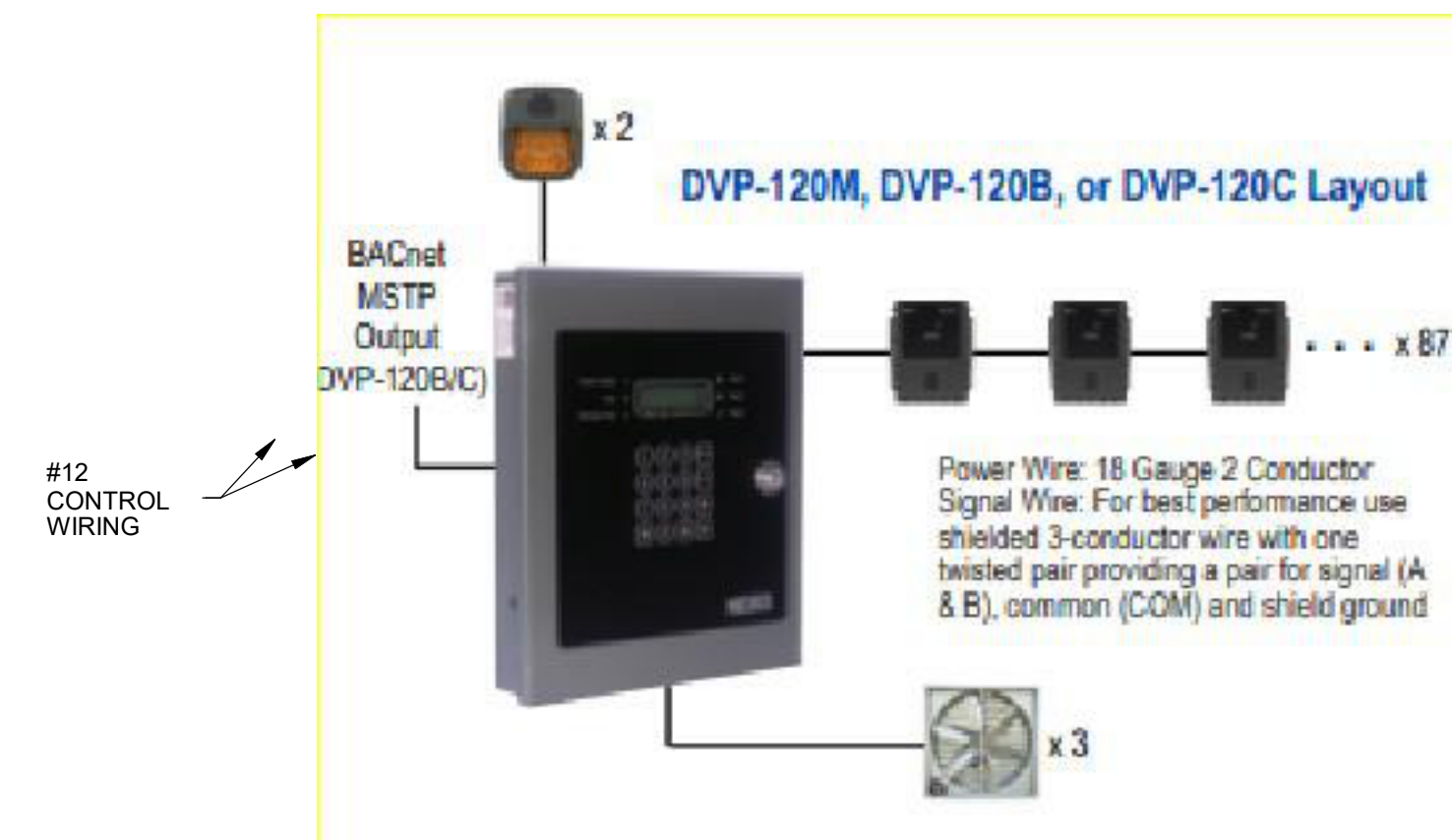
HANGAR CONTROLS DETAIL SCALE: NONE 2
