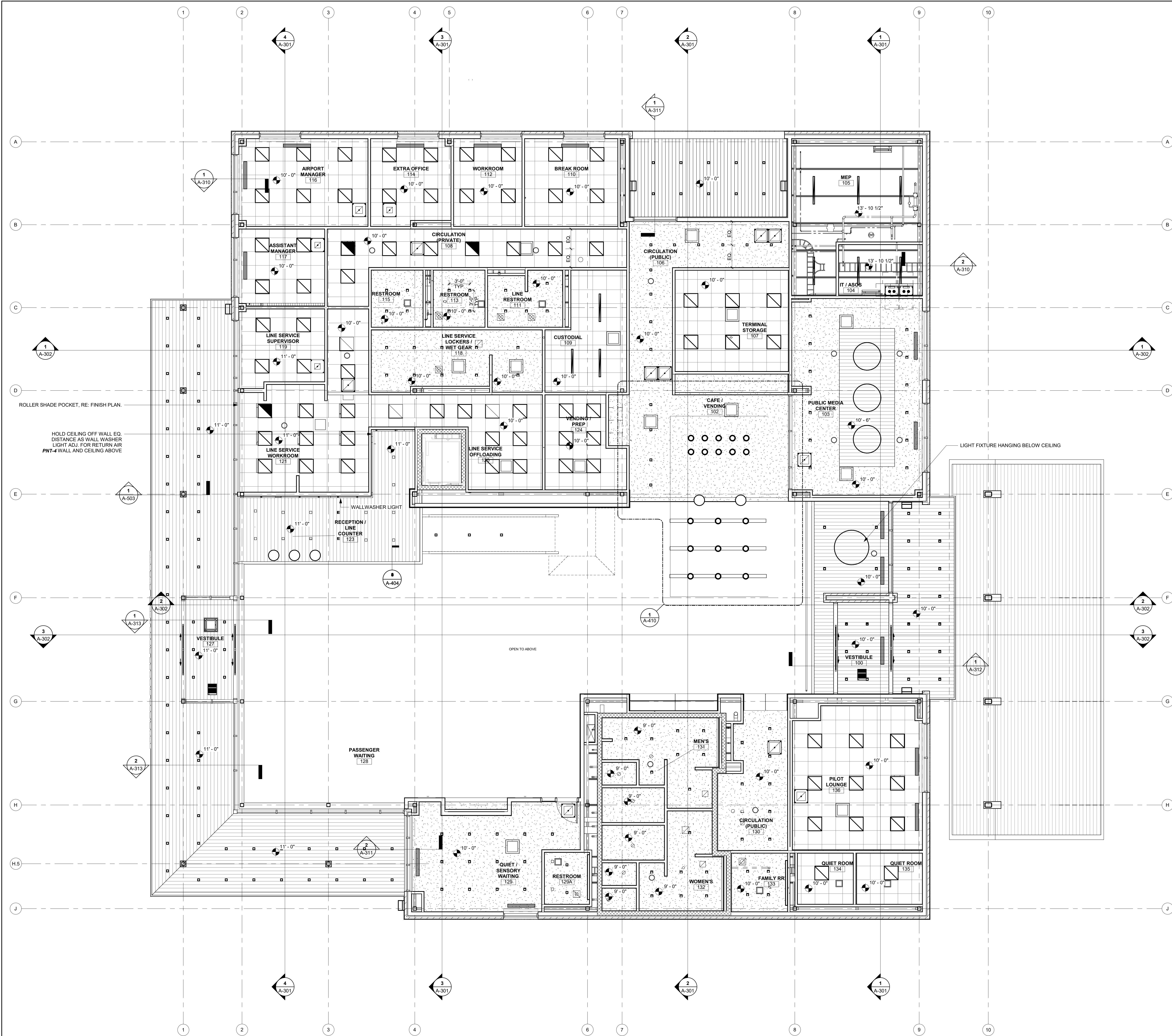
LOW REFLECTED CEILING PLAN 3/16" = 1'-0"
