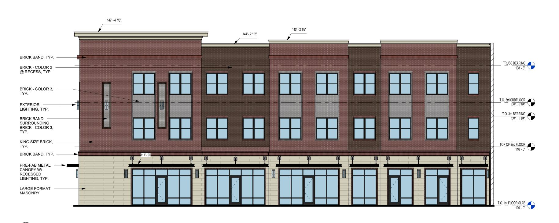
BRICK BAND, TYP. TRUSS BEARING 138' - 3" BRICK - COLOR 2 @ RECESS, TYP. T.O. 3rd SUBFLOOR 128' - 1 7/8" BRICK - COLOR 3, \_\_\_\_ TYP. T.O. 3rd BEARING 126' - 1 1/8" KING SIZE BRICK, TYP. TOP OF 2nd FLOOR 116' - 0" BRICK BAND, TYP. PRE-FAB METAL CANOPY W/ RECESSED LIGHTING, TYP. **EXTERIOR** LIGHTING, TYP. LARGE FORMAT MASONRY T.O. 1st FLOOR SLAB 100' - 0"
