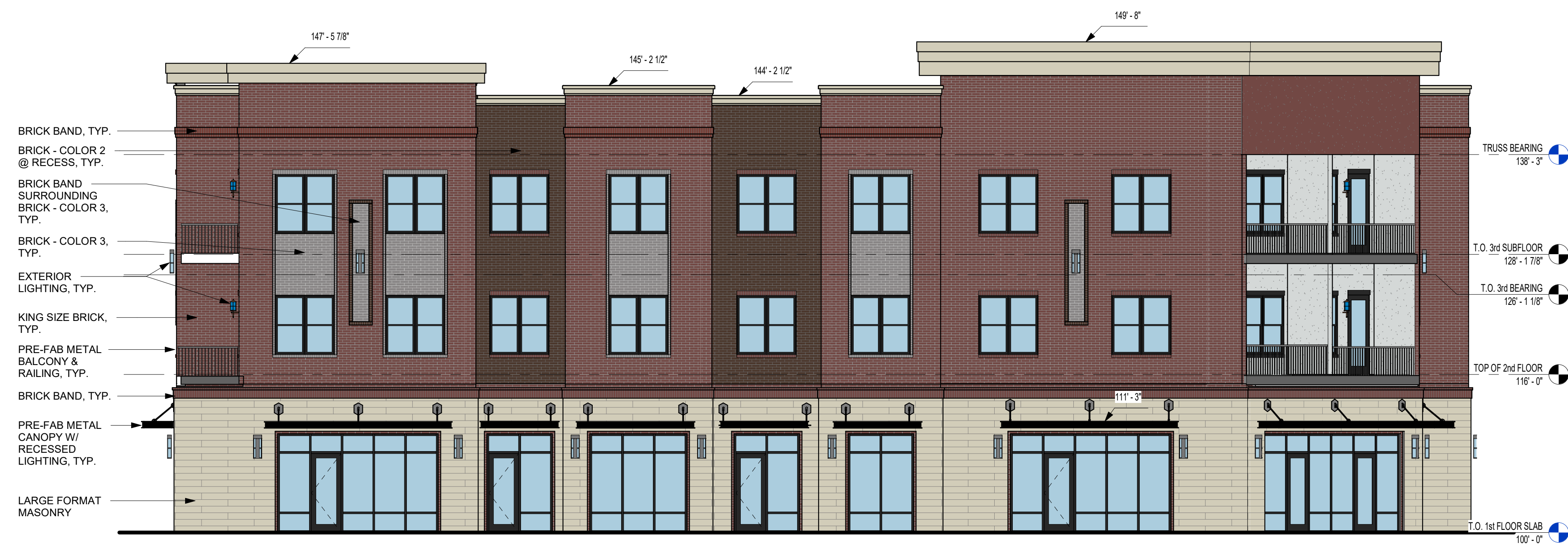
1 SOUTH ELEVATION - COLOR 1/8" = 1'-0"
