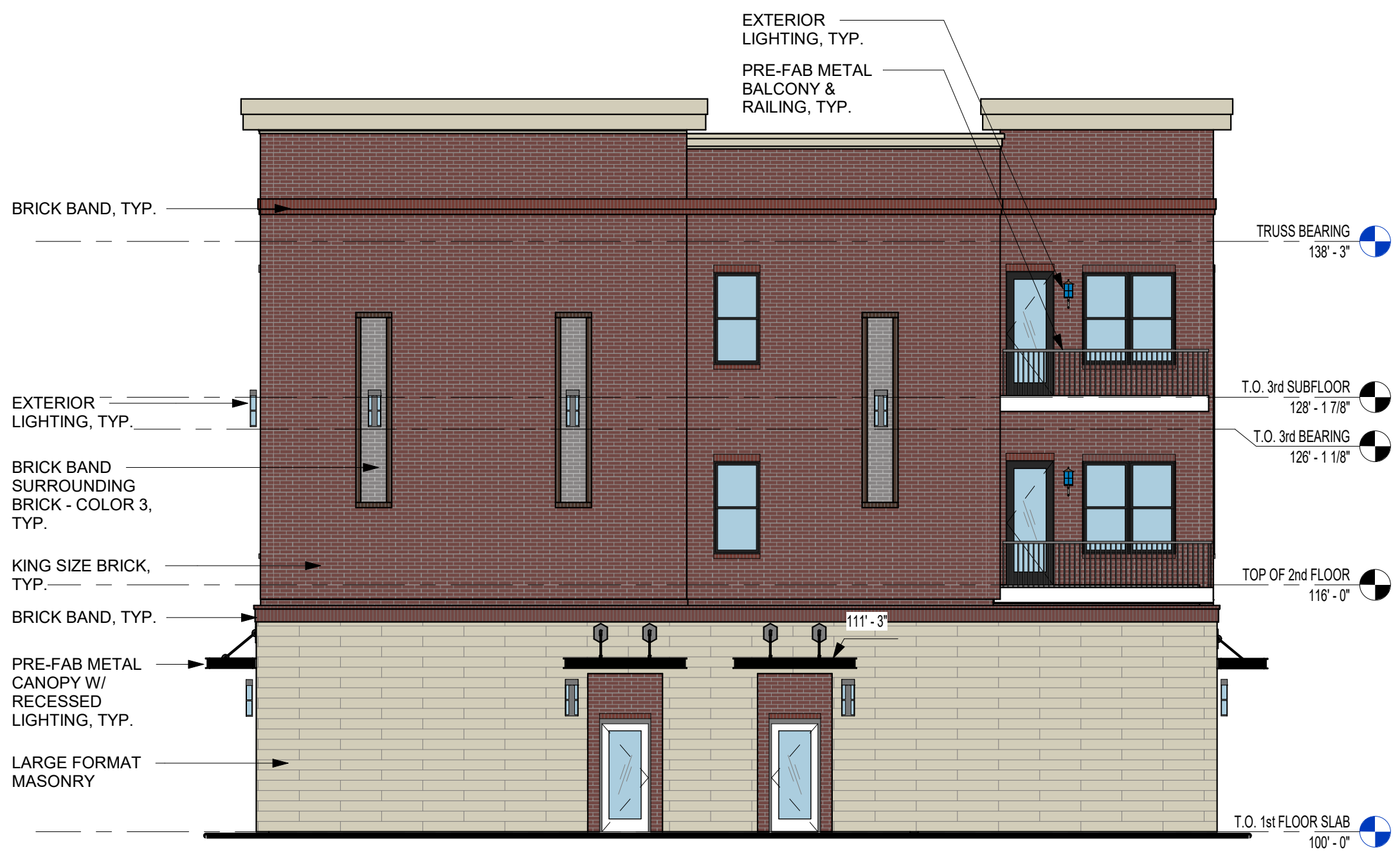
2 WEST ELEVATION 1 - COLOR 1/8" = 1'-0"
