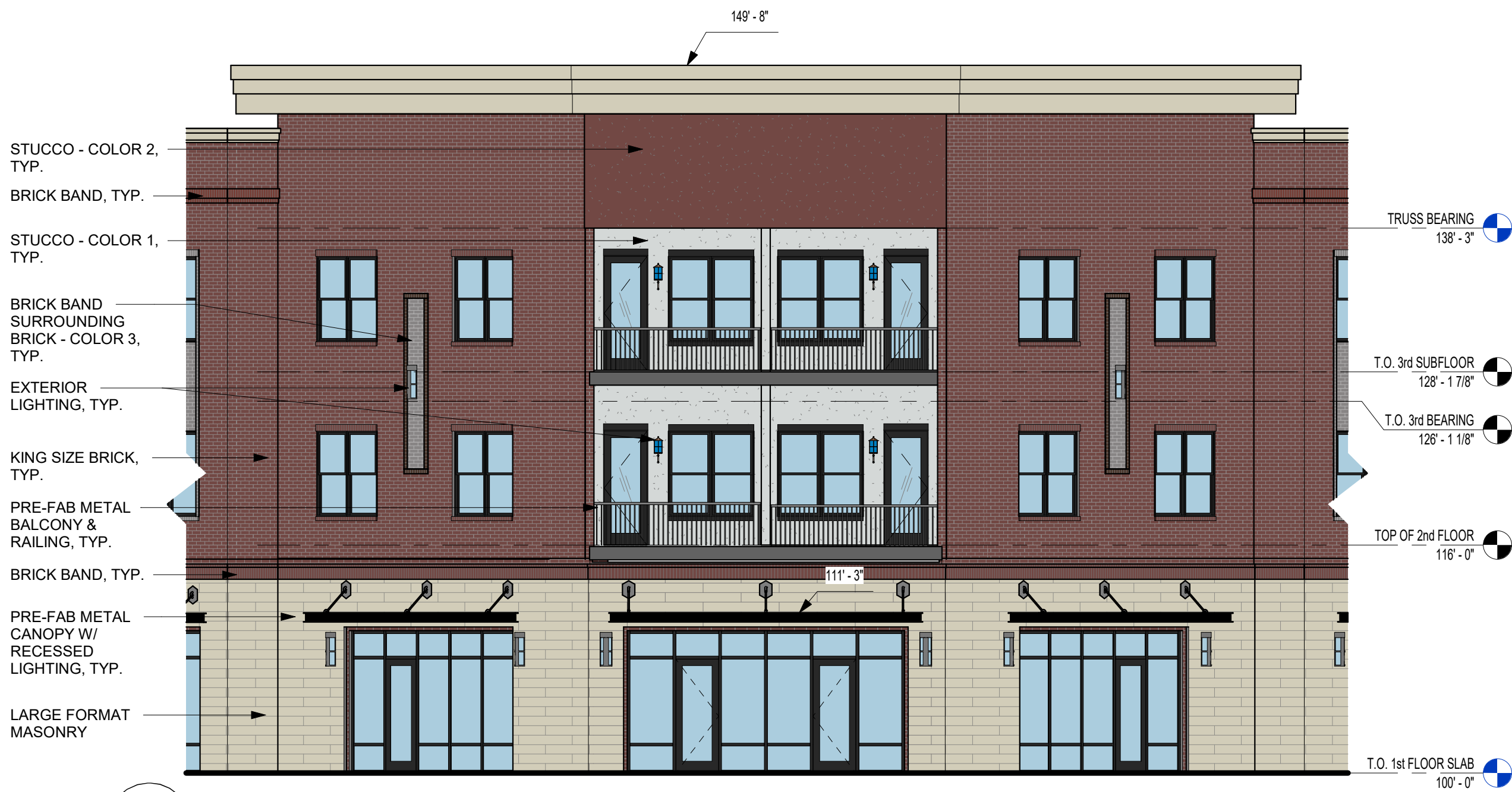
3 CORNER ELEVATION - COLOR 1/8" = 1'-0"
