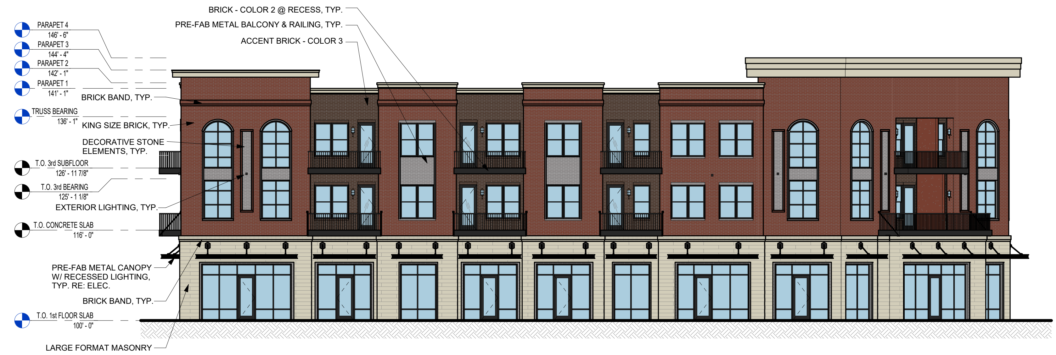
2 WEST ELEVATION - COLOR 3/32" = 1'-0"
