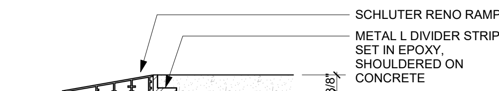
SEALED CONCRETE TO EPOXY TERRAZZO 6" = 1'-0" 7
