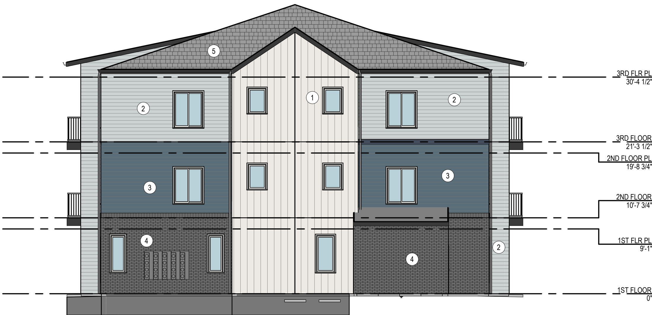
3 CLUBHOUSE - SIDE ELEVATION (BUILDING #5, TYPE C) 1/8" = 1'-0"
