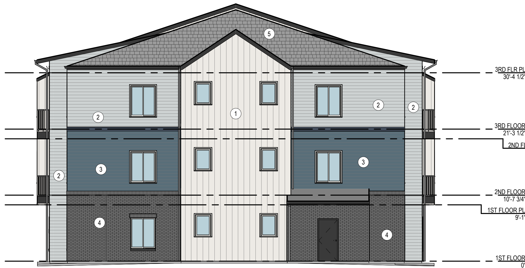
4 BUILDING TYPE A - LEFT ELEVATION (BUILDING #3 & #4) 1/8" = 1'-0"
