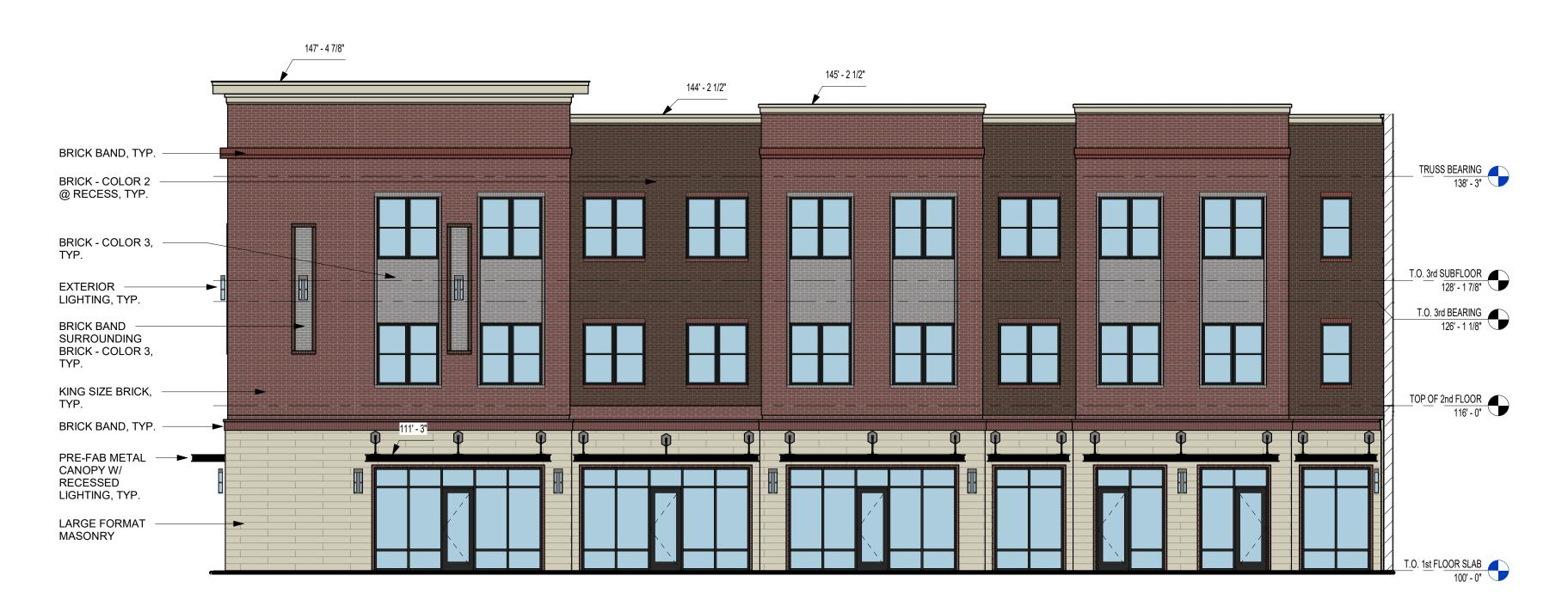
BRICK BAND, TYP. TRUSS BEARING 138' - 3" BRICK - COLOR 2 @ RECESS, TYP. T.O. 3rd SUBFLOOR 128' - 1 7/8" BRICK - COLOR 3, \_\_\_\_ TYP. T.O. 3rd BEARING 126' - 1 1/8" KING SIZE BRICK, TYP. TOP OF 2nd FLOOR 116' - 0" BRICK BAND, TYP. PRE-FAB METAL CANOPY W/ RECESSED LIGHTING, TYP. **EXTERIOR** LIGHTING, TYP. LARGE FORMAT T.O. 1st FLOOR SLAB 100' - 0" MASONRY
