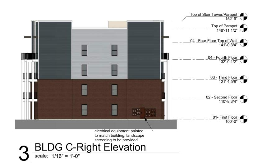
–All mech. equip. for building type C will be on roof. Roof
