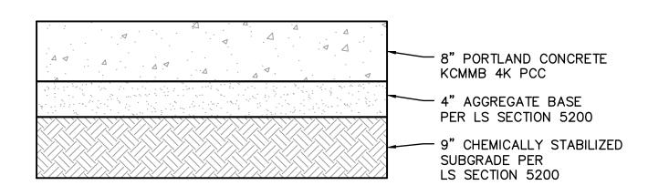
COMMERCIAL DRIVE PAVEMENT SECTION NOT TO SCALE
