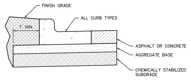
TYPICAL SUBGRADE PLACEMENT UNDER CURB
