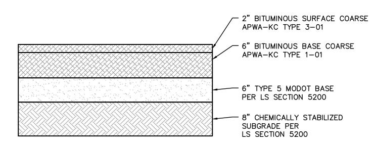
ASPHALT PAVEMENT (HEAVY TRAFFIC) WITH AGGREGATE BASE SECTION NOT TO SCALE
