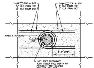
TYPICAL ROUND FIXED STRUCTURE PLAN DETAIL
