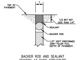
BACKER ROD AND SEALANT SECTION AT FIXED STRUCTURE
