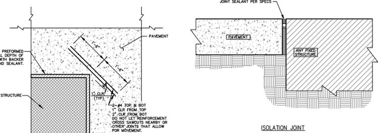
TYPICAL RECTANGULAR FIXED STRUCTURE PLAN DETAIL
