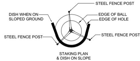
**STAKING PLAN & DISH ON SLOPE**
