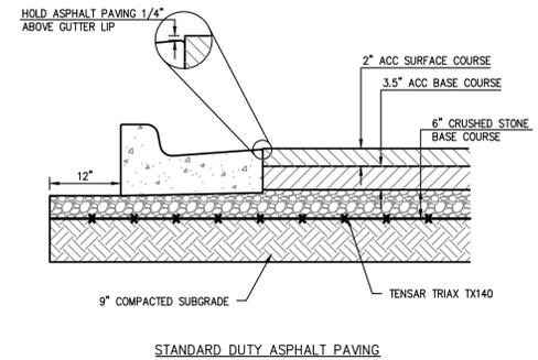
STANDARD DUTY ASPHALT PAVING
