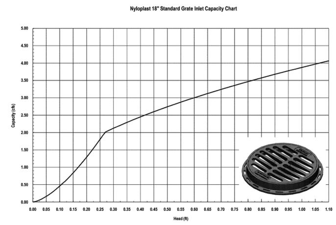
ALL SECONDARY STORM INLETS WILL CAPTURE 0.01-0.03 ACRES OF RUNOFF RESULTING IN < 0.5 CFS DURING THE 100-YEAR STORM. THIS WILL RESULT IN LESS THAN 0.1 FT OF HEAD OVER THE INLET PER THE CAPACITY CALCULATION ABOVE.
