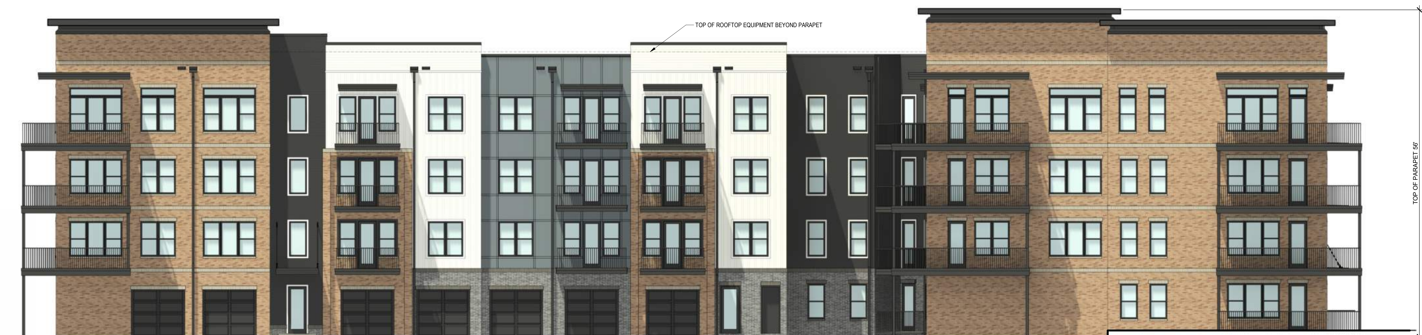
1 BUILDING B - REAR ELEVATION 1/8" = 1'-0"
