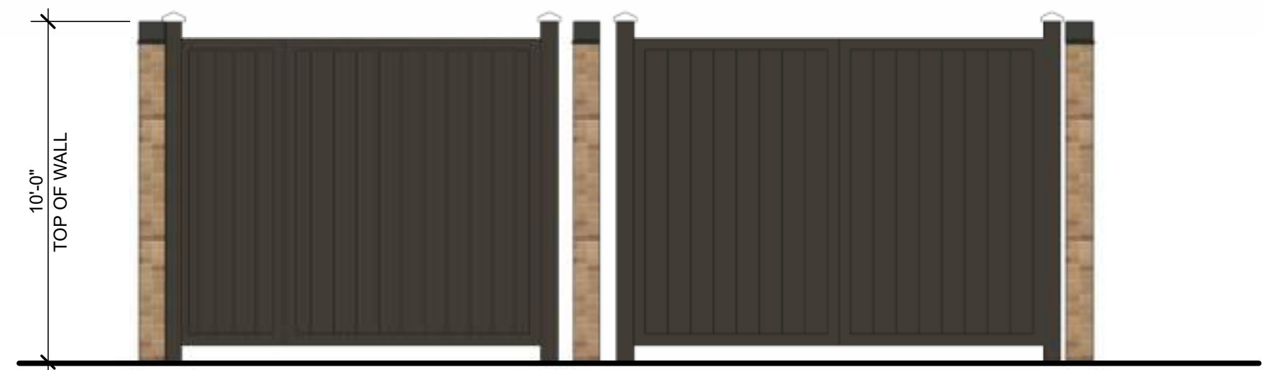
2 TRASH ENCLOSURE - FRONT ELEVATION 1/4" = 1'-0"
