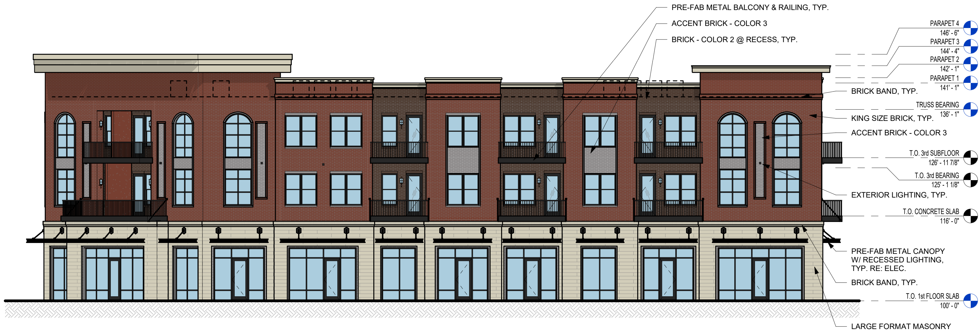
2 WEST ELEVATION - COLOR 3/32" = 1'-0"
