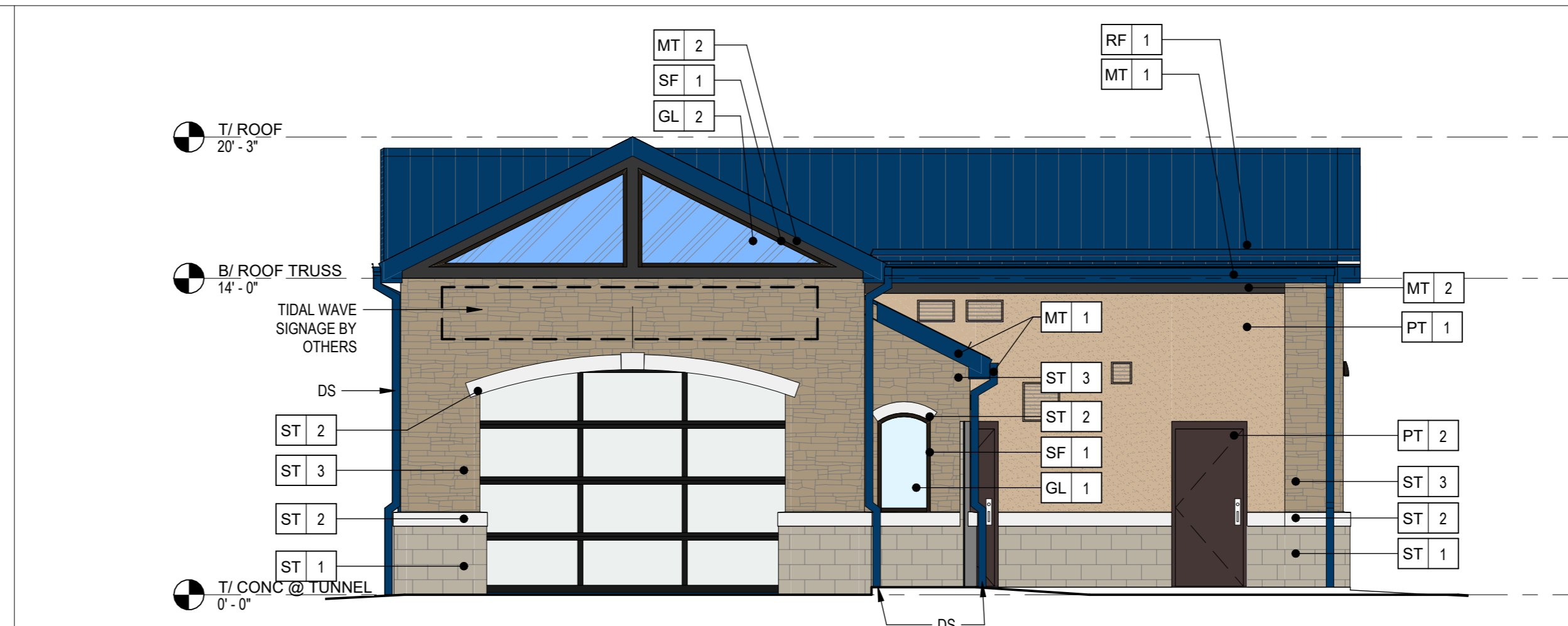
9G EXTERIOR ELEVATION - ENTRY A803 3/16" = 1'-0"
