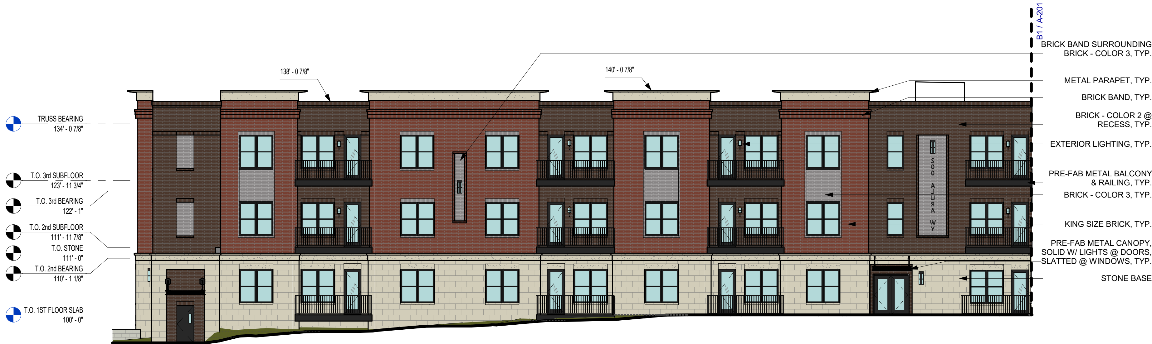
B2 COURTYARD SOUTH ELEVATION 3/32" = 1'-0"
