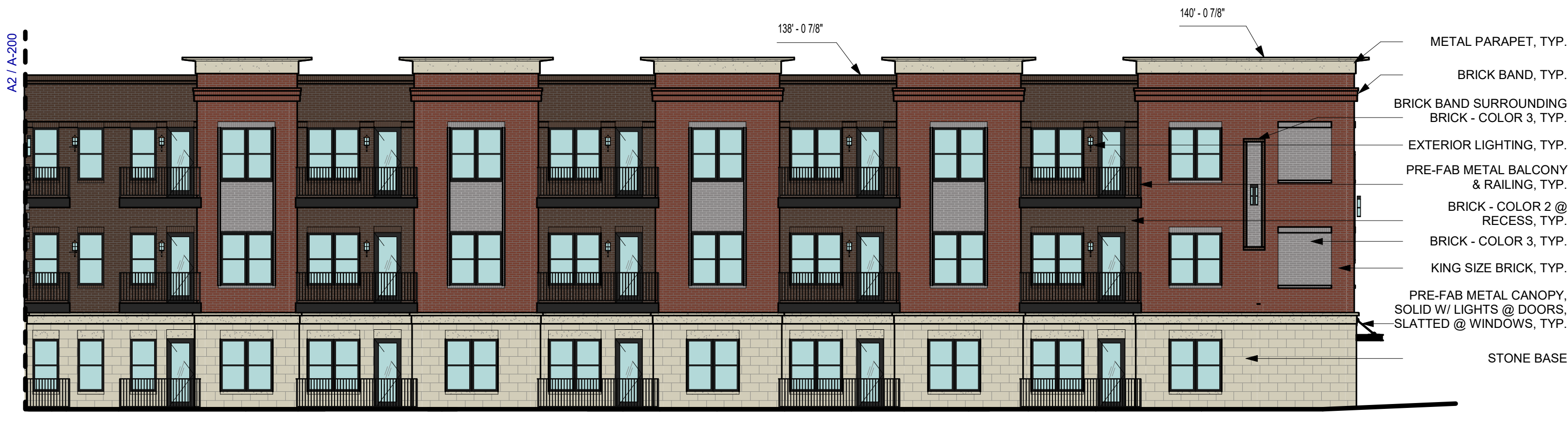
A1 COURTYARD WEST ELEVATION 3/32" = 1'-0"
