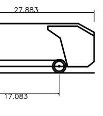
Hino 338 M + Wayne Royal GT14 Refuse Truck Overall Length 27.883ft Overall Width 8.042ft Overall Body Height 10.488ft Min Body Ground Clearance 1.318ft Track Width 8.042ft Lock-to-lock time 6.00s Curb to Curb Turning Radius 27.400ft
