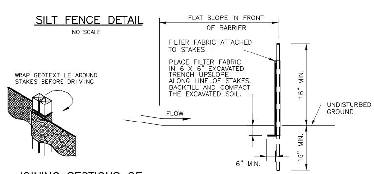
JOINING SECTIONS OF SILT FENCE DETAIL NO SCALE
