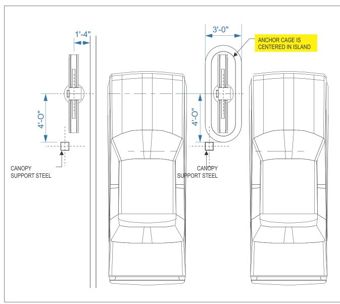
CHANDLER SIGNS TO PROVIDE ORDERING STATIONS. CHANDLER SIGNS TO PROVIDE TEMPLATES AND ANCHOR BOLTS. GEN. CONTRACTOR TO SET ANCHOR BOLTS AND POUR CONCRETE. CHANDLER SIGNS TO INSTALL ORDERING STATIONS.
