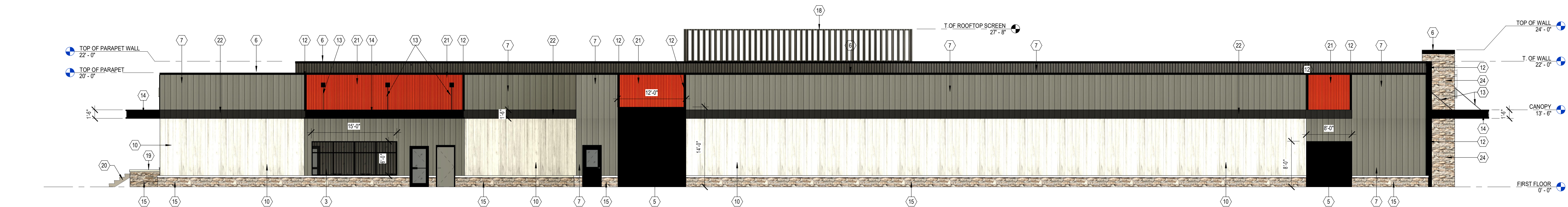
3 NORTH ELEVATION SCALE: 1/8" = 1'-0" METAL PANELS: 2,154 S.F. (43%) FAUX FIBER CEMENT: 1,560 S.F. (31%) THIN STONE VENEER: 861 S.F. (17%) WINDOWS/DOORS: 385 S.F. (9%) FACADE TOTAL: 4,960 S.F. (100%)
