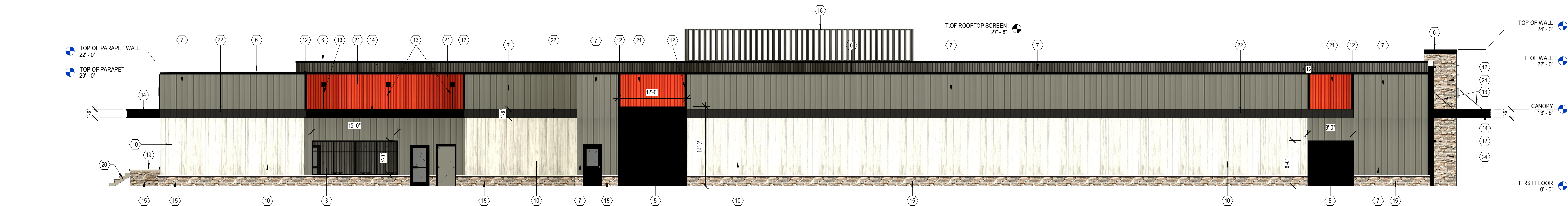
3 NORTH ELEVATION SCALE: 1/8" = 1'-0" METAL PANELS: 2,154 S.F. (43%) FAUX FIBER CEMENT: 1,560 S.F. (31%) THIN STONE VENEER: 861 S.F. (17%) WINDOWS/DOORS: 385 S.F. (9%) FACADE TOTAL: 4,960 S.F. (100%)
