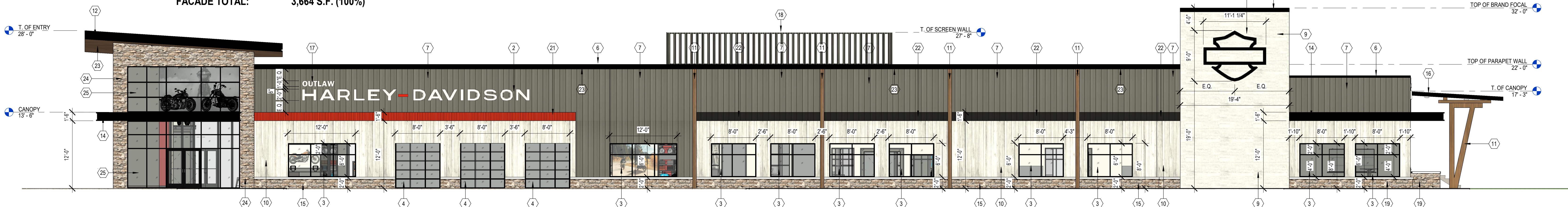
2 SOUTH ELEVATION SCALE: 1/8" = 1'-0" METAL PANELS: 1,739 S.F. (33%) FAUX FIBER CEMENT: 1,634 S.F. (32%) THIN STONE VENEER: 545 S.F. (11%) WINDOWS/DOORS: 1,260 S.F. (24%) FACADE TOTAL: 5,178 S.F. (100%)
