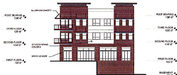
2 BLDG 4 SOUTH ELEVATION 3/32" = 1'-0"
