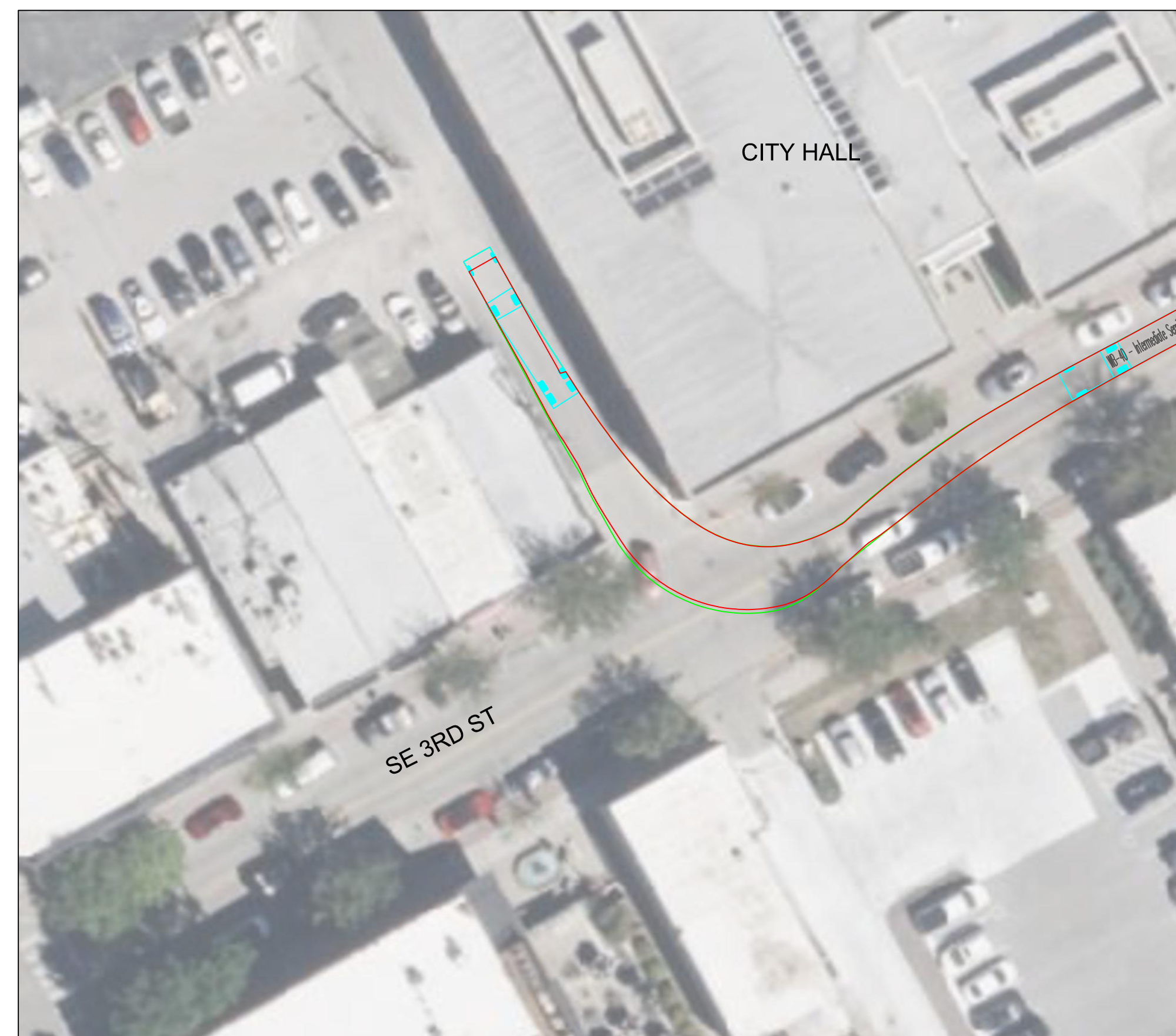
INBOUND RIGHT TURN FROM SE 3RD ST TO THE ALLEY
