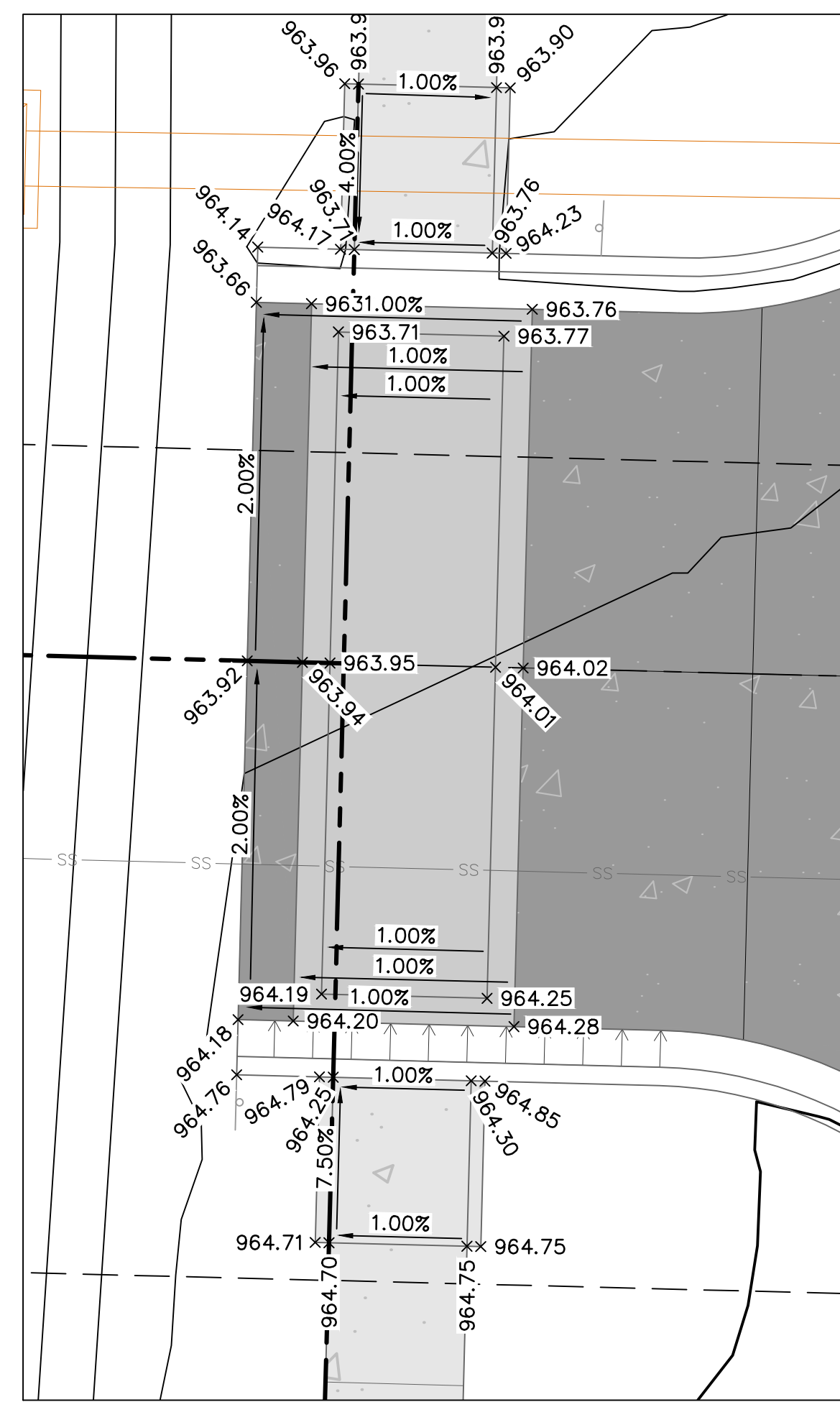
SIDEWALK RAMP DETAIL B SCALE: 1" = 5'
