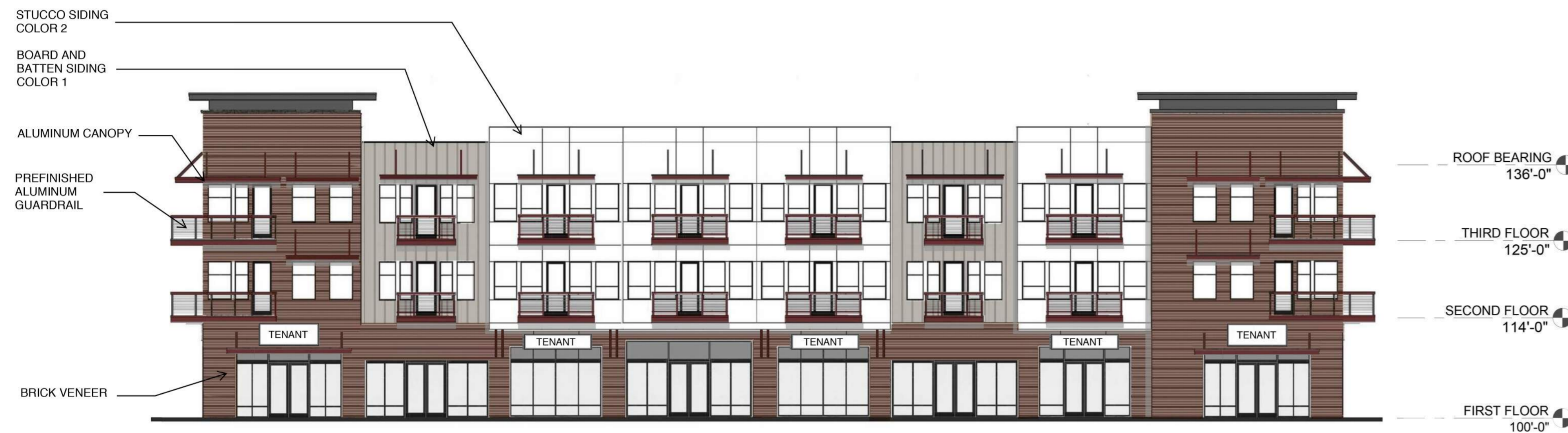
3 BLDG 4 NORTH ELEVATION 3/32" = 1'-0"
