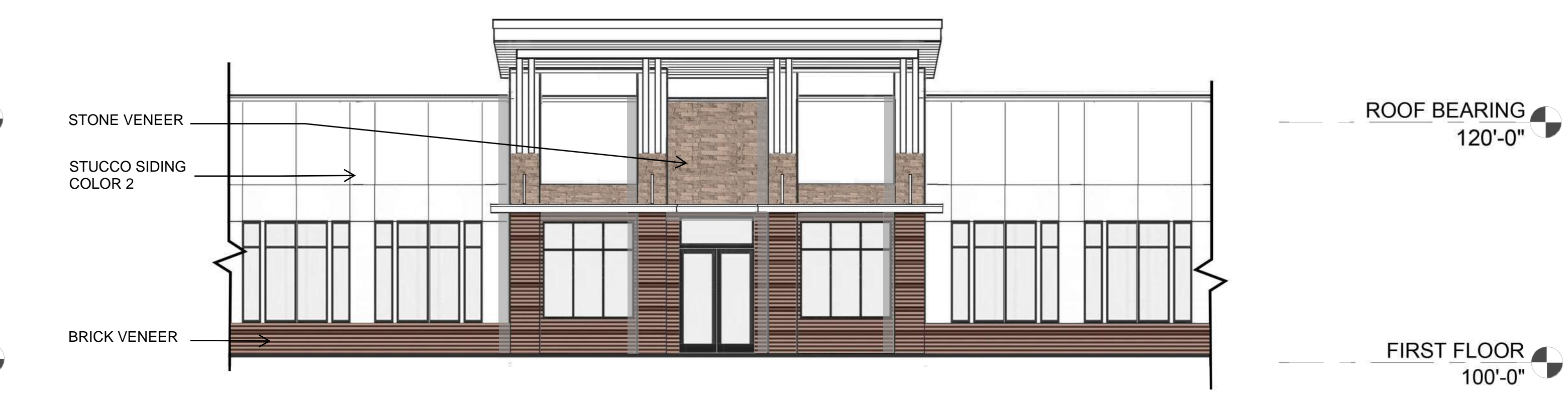
1 TYPICAL ENTRY NORTH ELEVATION 1/8" = 1' -0"
