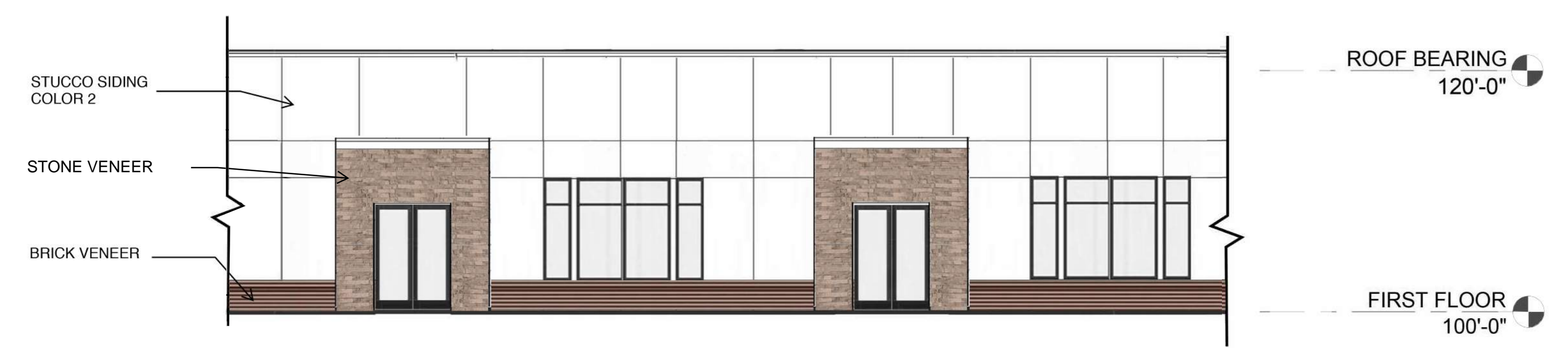
3 TYPICAL REAR SOUTH ELEVATION 1/8" = 1' -0"
