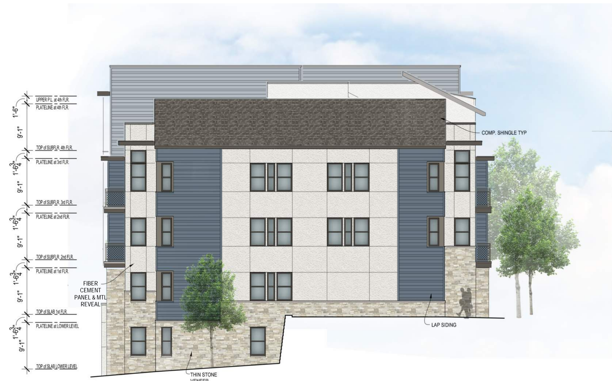
APARTMENT BLDG LEFT ELEVATION 3/32" = 1'-0"
