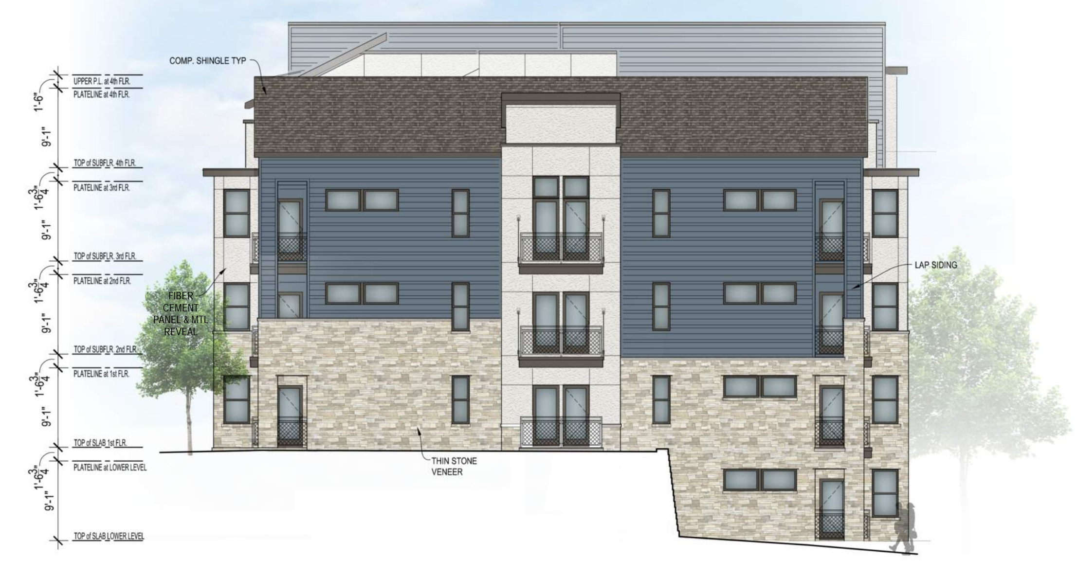
APARTMENT BLDG RIGHT ELEVATION 3/32" = 1'-0"
