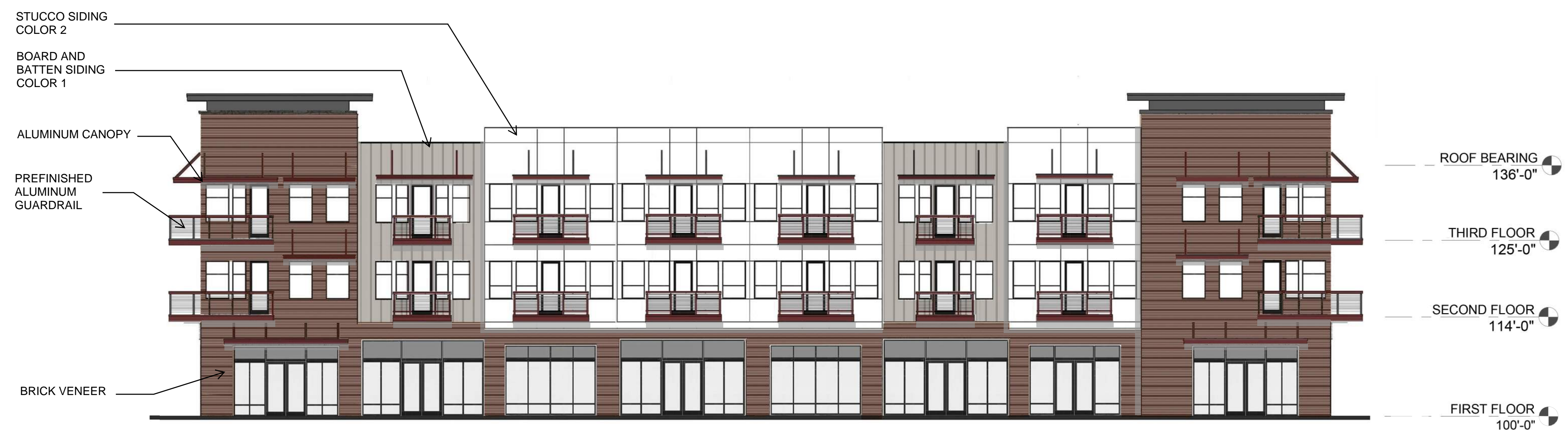
3 BLDG 4 NORTH ELEVATION 3/32" = 1'-0"
