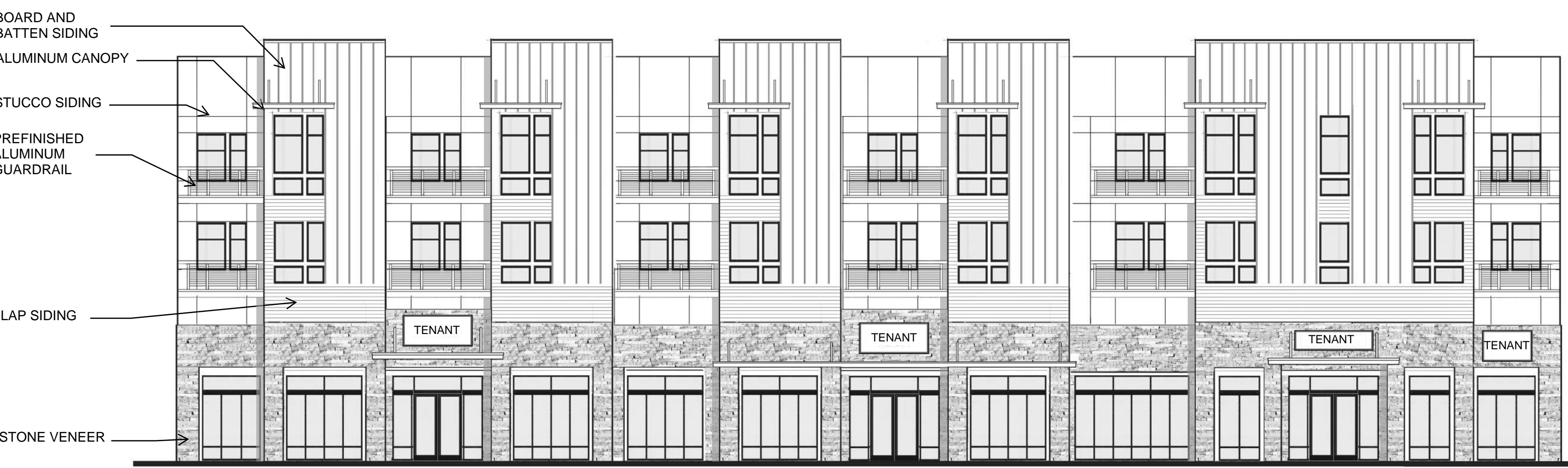
3 BLDG 5 NORTH ELEVATION 3/32" = 1' - 0"
