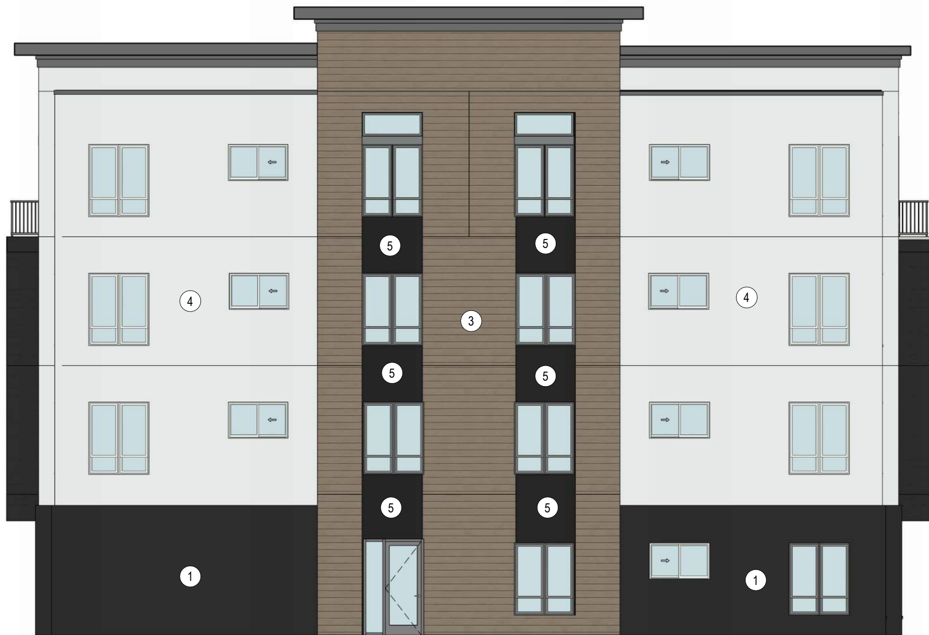
1 BUILDING 1 - WEST ELEVATION 1/8" = 1'-0"
