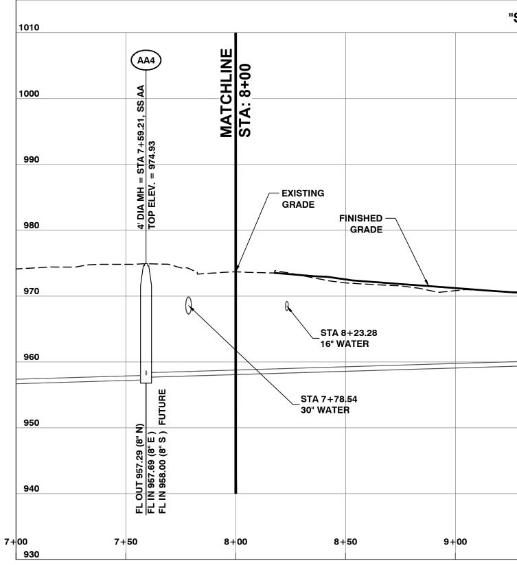
NOTE: FUTURE FLOWLINES SHOWN FOR REFERENCE ONLY. FUTURE CONNECTIONS TO BE CORE DRILLED.
