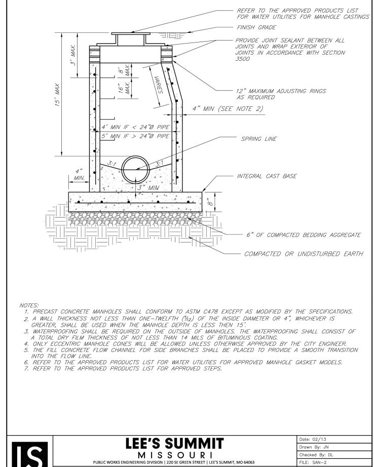
STANDARD PRECAST MANHOLE - SANITARY SEWER
