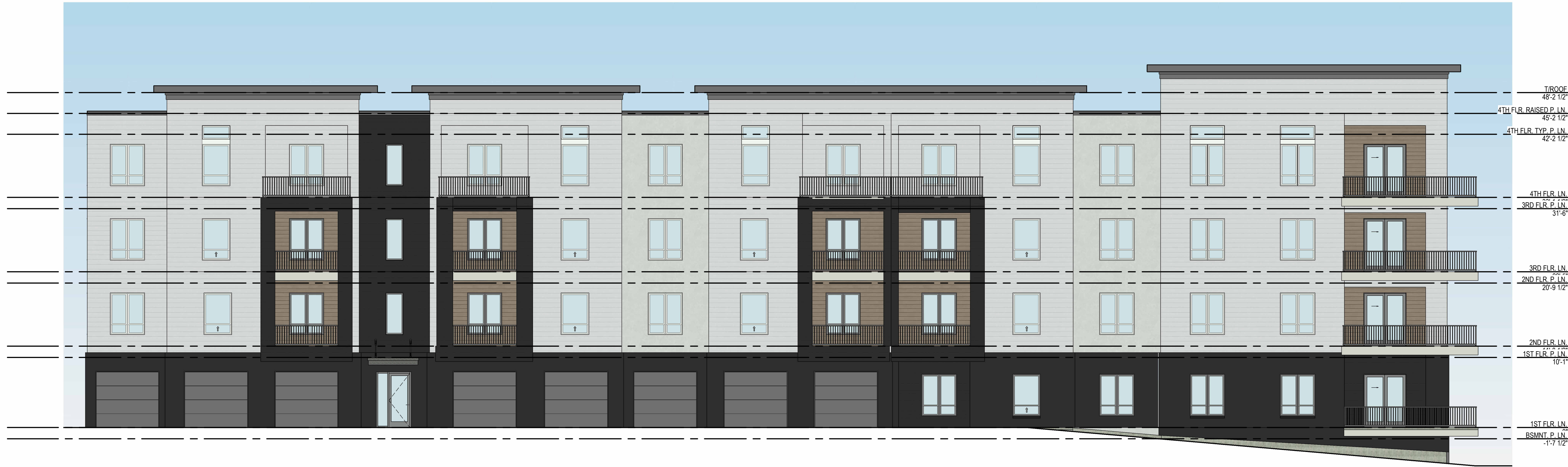
1 BUILDING 2 - EAST ELEVATION 1/8" = 1'-0"
