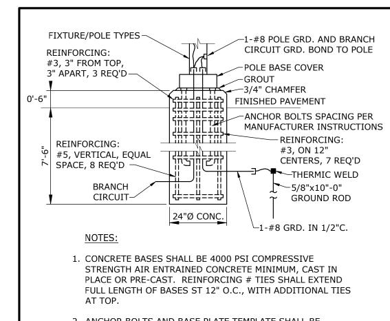
2. ANCHOR BOLTS AND BASE PLATE TEMPLATE SHALL BE PROVIDED BY LIGHTING POLE MANUFACTURER TO VENDOR FOR BASES PRIOR TO CONSTRUCTION.
