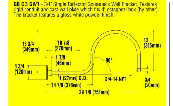
GB D 3 GWT - 3/4" Single Reflector Gooseneck Wall Bracket. Features rigid conduit and cast wall plate which fits 4" octagonal box (by other). The bracket features a gloss white powder finish.
