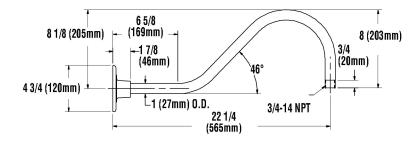
GB B 3 GWT - 3/4" Single Reflector Gooseneck Wall Bracket. Features rigid conduit and cast wall plate which fits 4" octagonal box (by other). The bracket features a gloss white powder finish.
