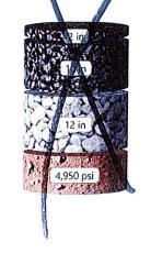
Total HMA thickness should be within the same range on both pavement sections for accurate comparison 2-3 in | 3-6 in | 6-14 in
