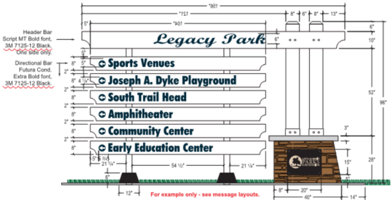
Figure 4 - Typical specification of proposed ground signs
