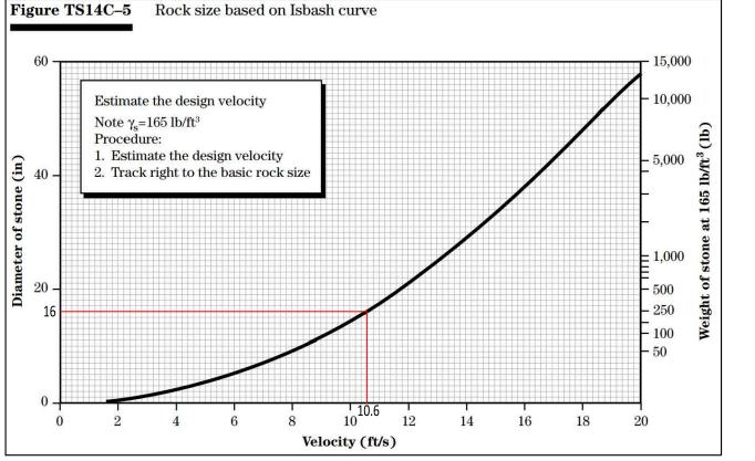
MAXIMUM 100-YR OUTLET VELOCITY PER DRAINAGE CALCULATIONS (SHEET C202) ≈ 10.6 FT/S.
