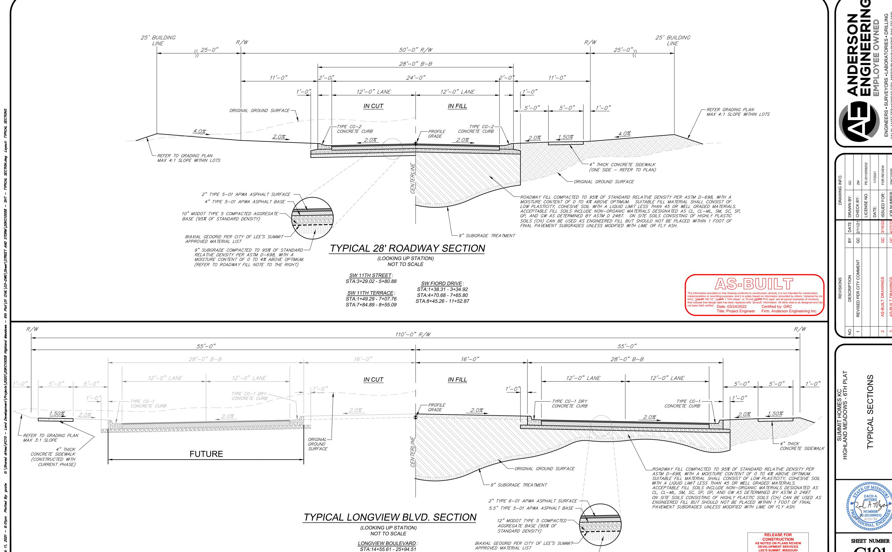
9" SUBGRADE COMPACTED TO 95% OF STANDARD-
