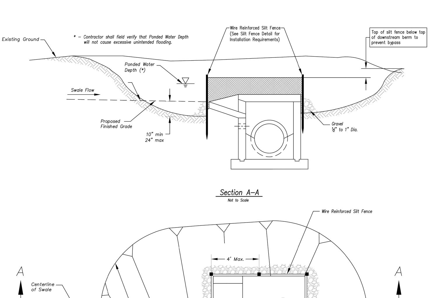
Excavated Area for Sediment Storage — Limits of Excavation ½" to 1" Dia. <u>Notes:</u>
