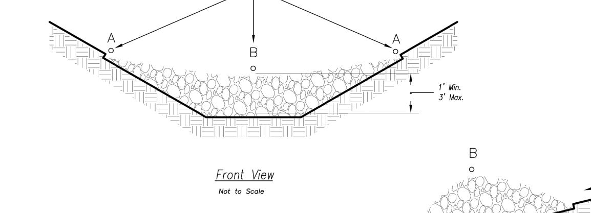
Elevation at end Points "A" must be minimum 6" higher than elevation of flow line at point "B"
