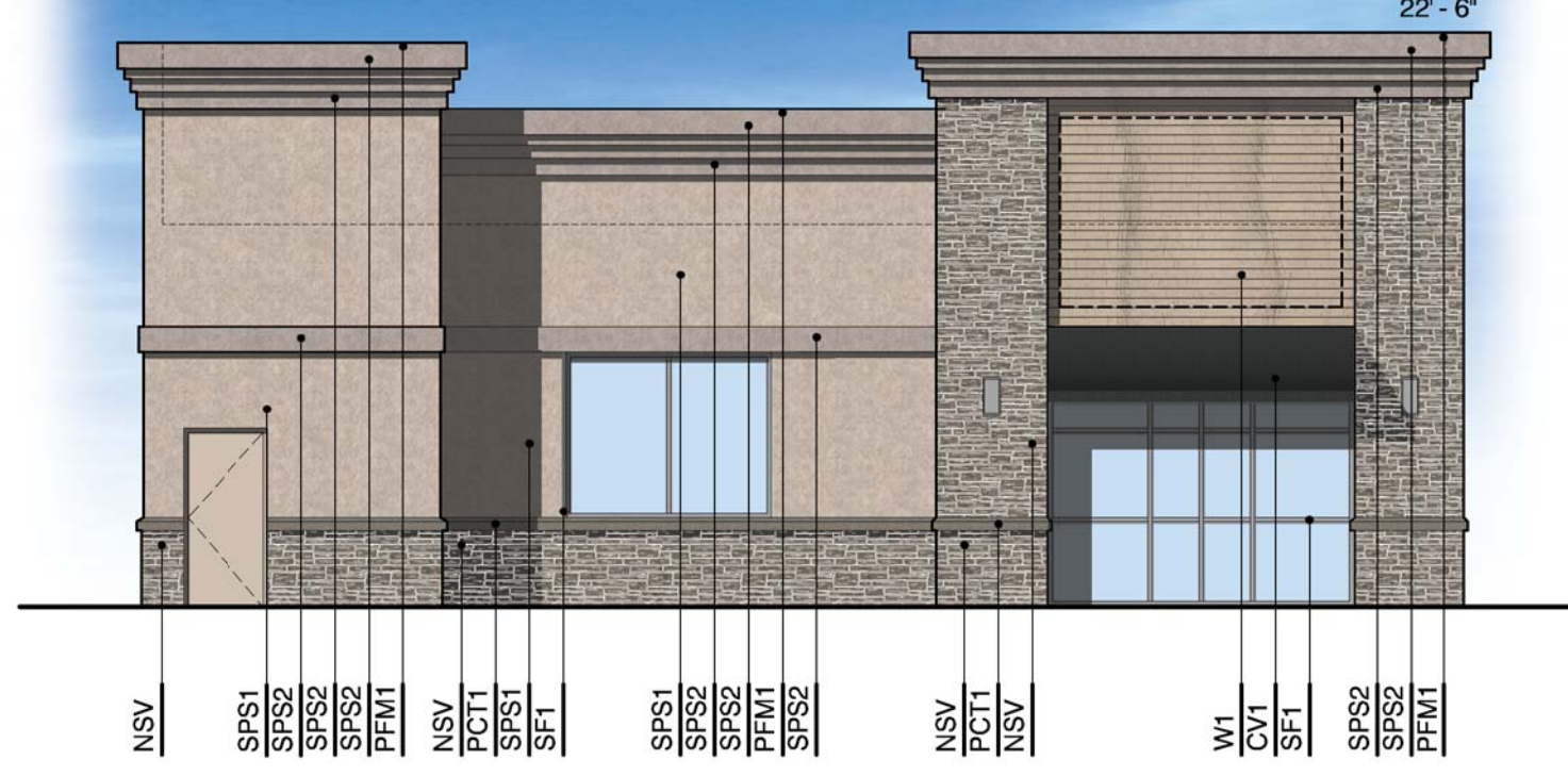
proposed North Elevation 1/8" = 1'-0"
