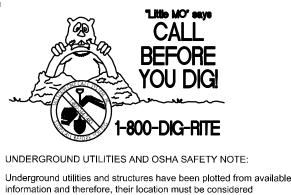
information and therefore, their location must be considered approximate only. It is the responsibility of the individual contractors to notify the utility companies before actual construction. All O.S.H.A rules and regulations established for the type of construction required by these plans shall be strictly followed (ie. trenching, blasting, etc.)
