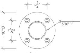
$10"Øx_8^{5"}$  STEEL PLATE W/ (4)  $\frac{5}{8}$ "Ø THREADED ANCHOR RODS MIN EMBED. = 24" INTO CONCRETE W/NUT/WASHER/NUT @ EMBED. END
