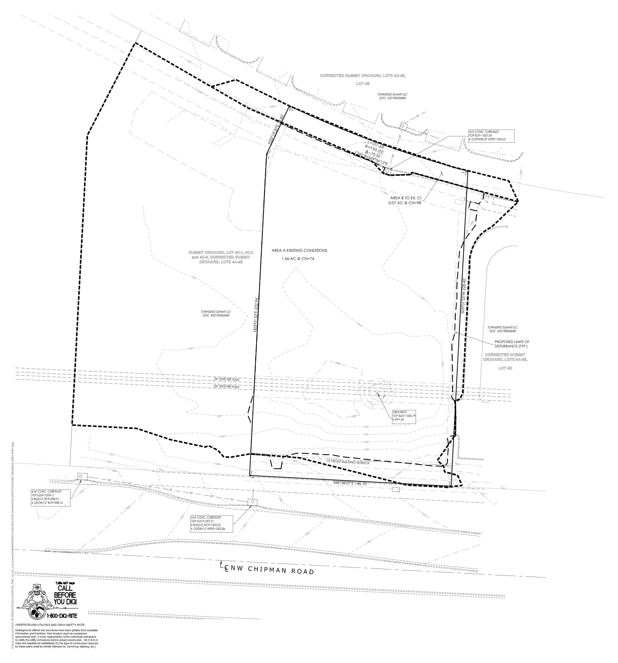
EX ID AREA A 2-Year 10-Year 100-Year 2-Year 10-Year 100-Year THIS PLAN IS FOR DRAINAGE PURPOSES AND REFERENCE ONLY. DO NOT USE FOR CONSTRUCTION. MINIMUM TIME OF CONCENTRATION = 5 MINUTES EXISTING SOILS TYPE = C CN PVMT = 98 CN GRASS = 74 CN COMMERCIAL AREAS = 94
