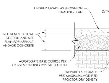
FLUSH PAVEMENT AT SIDEWALK RAMP
