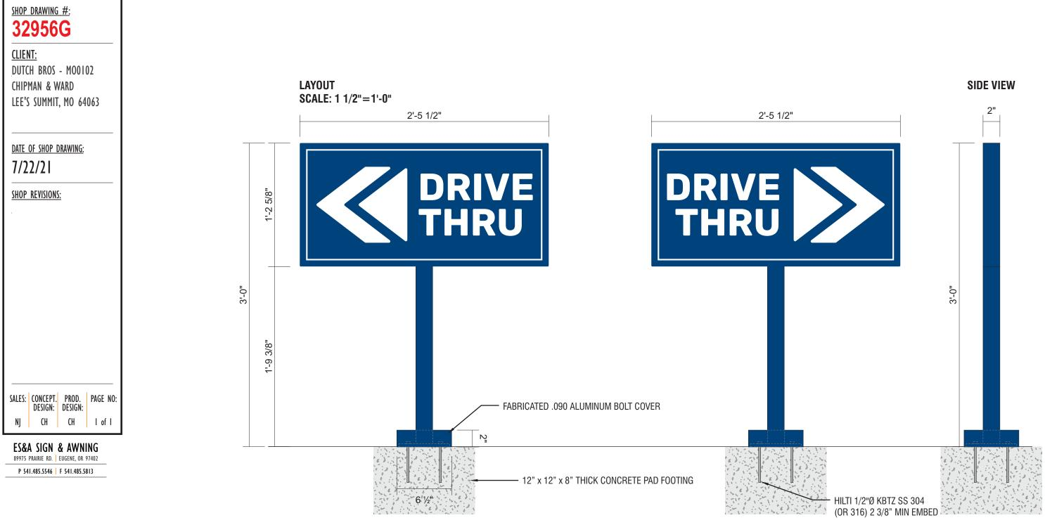
DIAMOND GRADE REFLECTIVE WHITE VINYL WITH DIGITALLY PRINTED PMS 541 C BLUE BACKGROUND 2" X 2" SQUARE TUBE ALUMINUM FRAME & POST WITH ALUMINUM FACES & 3/8" X 6" X 6" PLATE **FABRICATED .090 ALUMINUM BOLT COVER** PAINT PMS 541 C **INSTALL PLATE-MOUNT SIGN WITH HILTI KWIK BOLTS** PAD FOOTING INSTALLED BY GC
