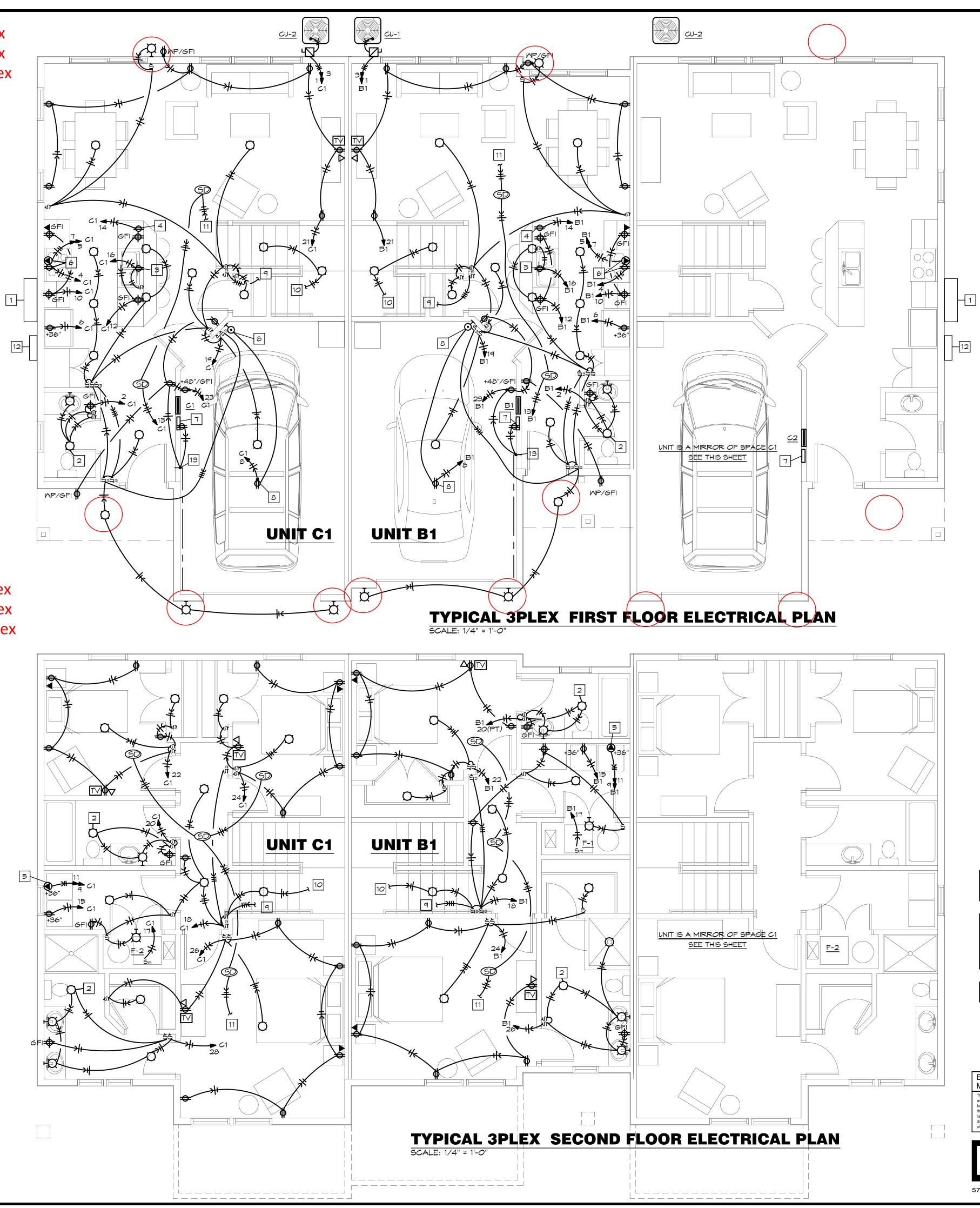
9 light fixtures on front of 3plex 12 light fixtures on front of 4plex 15 light fixtures on front of 5 plex
