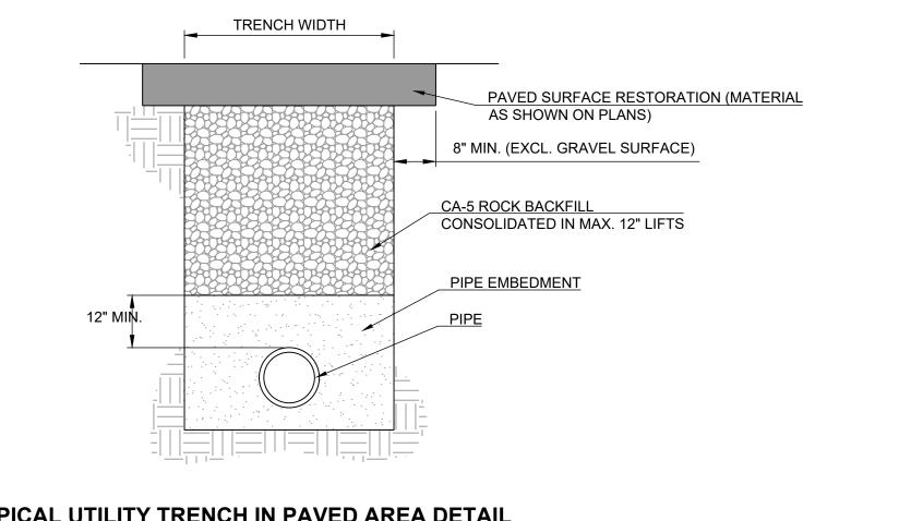
TYPICAL UTILITY TRENCH IN PAVED AREA DETAIL NOT TO SCALE
