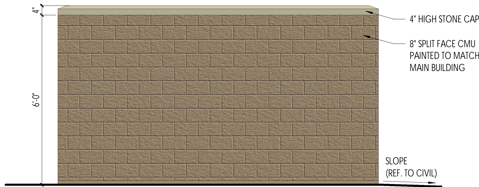
03 DUMPSTER ENCLOSURE SIDE ELEVATION SCALE: 1/2" = 1'-0"
