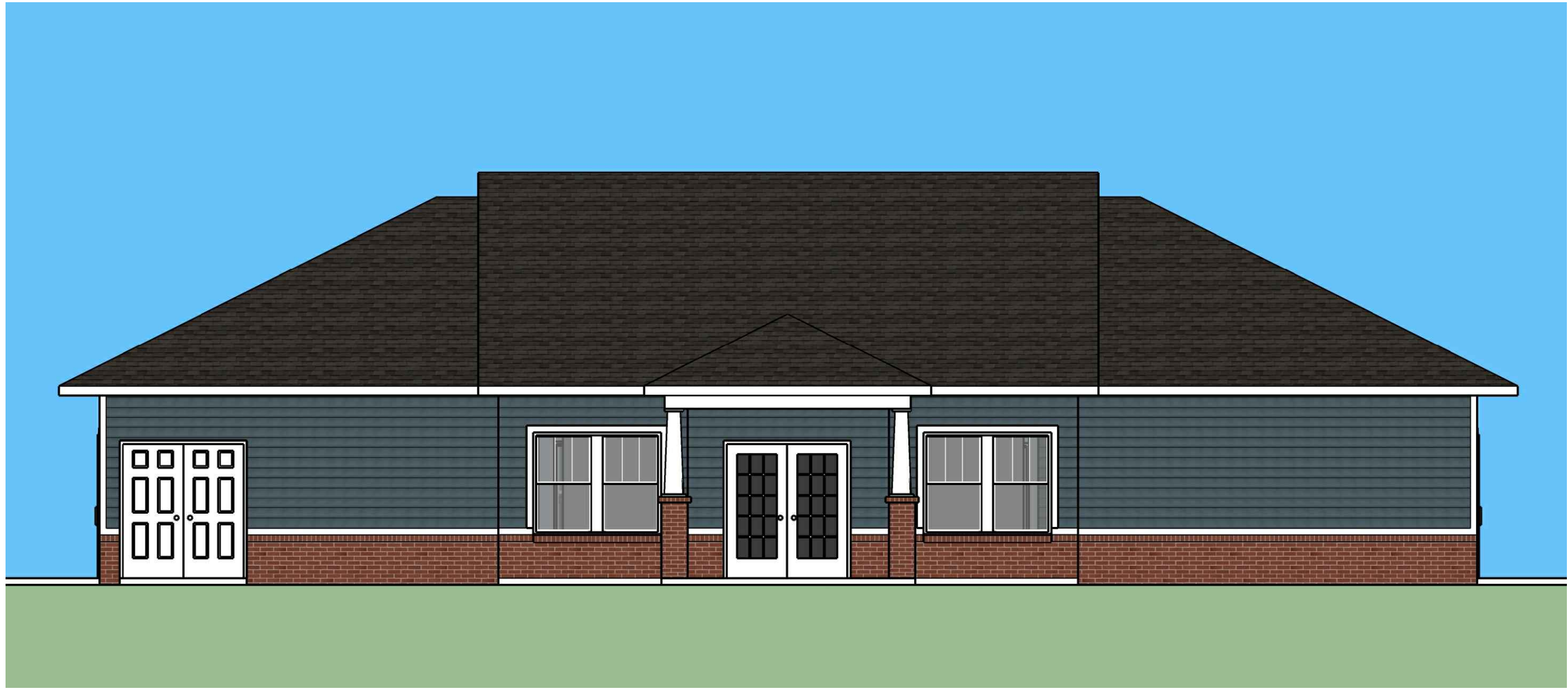
COMMUNITY BUILDING REAR ELEVATION SCALE: 3/16" = 1'-0"
