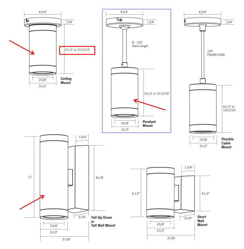
\*Wall mount cylinders include a 4-3/4"W x 5-1/8"H optional mounting plate for use with larger junction boxes.
