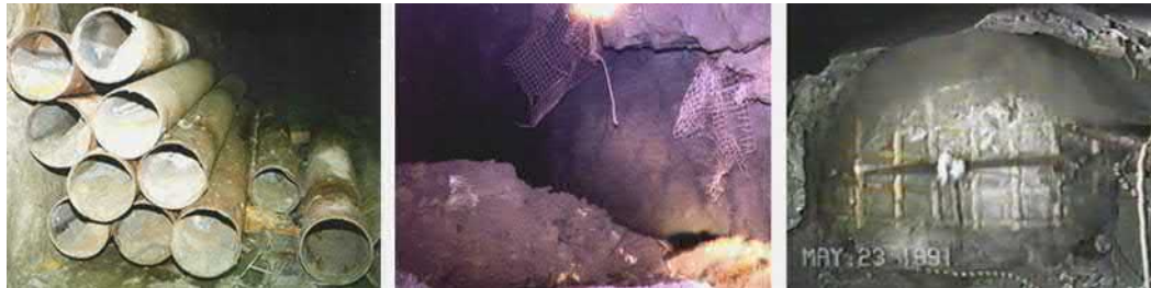
Figure 3. Common backfill system failures. From left to right, plug or burst pipelines, backfill sloughing and critical bulkhead failure.
