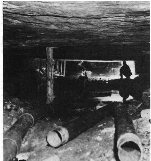
Fig. 6. Typical underground flushing pipeline for a controlled backfilling operation.
