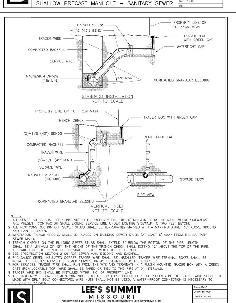
BUILDING SEWER STUB AND RISER
