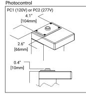
Photocontrol cover is precision machined from corrosion-resistant 6061-T6 aluminum and is secured to bollard head with tamper resistant stainless steel hardware. The photocontrol option is available in dedicated 120V or 208-277V. When specifying a photocontrol option make sure to designate the appropriate voltage within the catalog logic.
