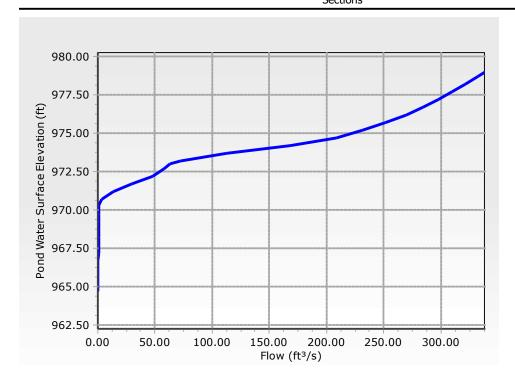
RATING TABLE FOR ONE OUTLET TYPE Structure ID = Culvert - 1 (Culvert-Circular)
