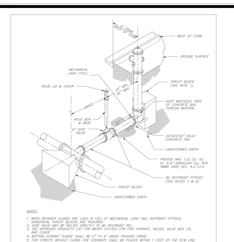
BUT NOT MORE THAN 10' FROM EDGE OF PAVEMENT. FIRE HYDRANT SHALL NOT BE PLACED IN
