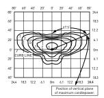
XSPW-B-\*\*-2ME-8L-40K-UL Mounting Height: 15' (4.6) A.F.G. Initial Delivered Lumens: 8,475 Initial FC at grade
