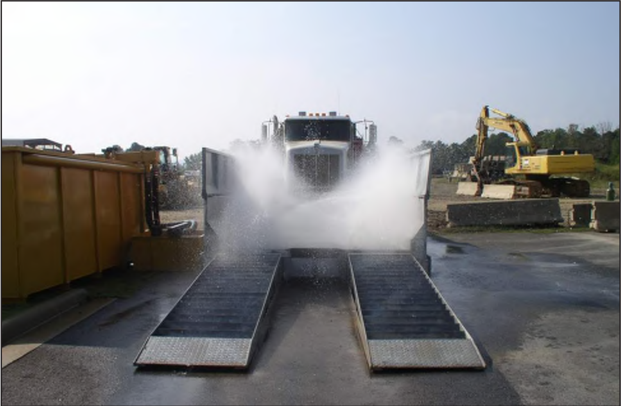
Figure 6.3 Industrial wheel wash unit with self contained and recycled wash water. Source: Innovative Equipment Solutions .
