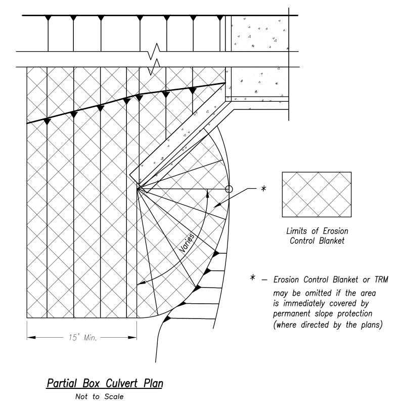
Installation Around Culvert Slope
