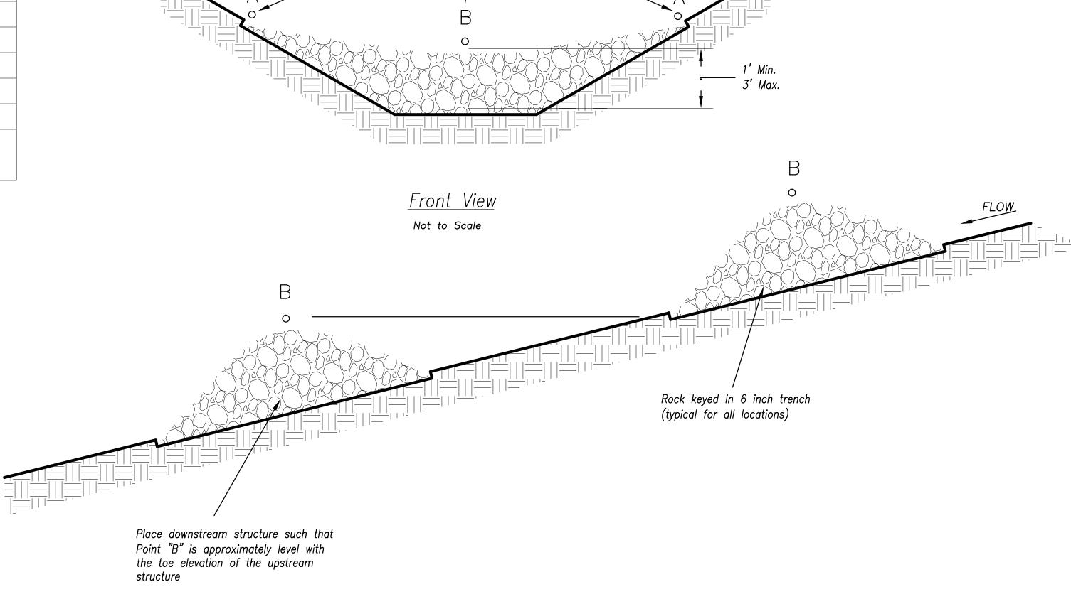
Elevation at end Points "A" must be minimum 6" higher than elevation of flow line at point "B"
